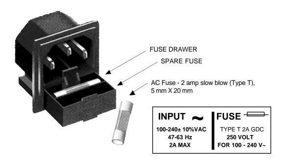
FIGURE 2.5 Fuse Location and Spare Fuse
