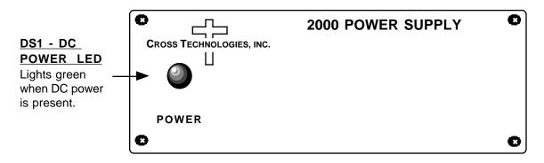
FIGURE 2.2 2000-01 Front Panel Indicator
