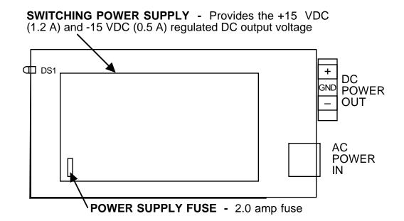
FIGURE 2.4 2000-01 On-Card AC Power Supply Fuse (See Section 2.4 for instructions on removing the unit from the extrusion)
